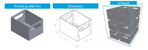
Figure 2: Example of packing density optimization: Box original design and number of parts that fit in the print bed. Data courtesy of Henkel AG & Co. KgaA
