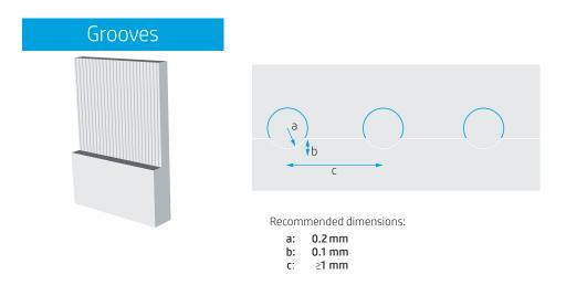
Figure 13: Grooves to increase bonding area: Design recommendations
