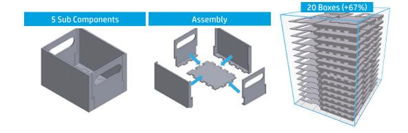
Figure 3: Example of split part to optimize packing density: With the split, the packing density increased by 67%. Data courtesy of Henkel AG & Co. KgaA
